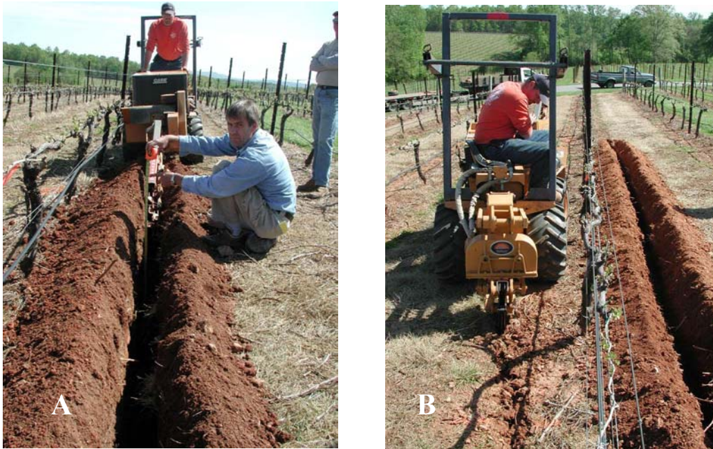
Figure 1. Gill Giese is measuring depth of trench used to prune Cabernet Sauvignon roots at Shelton Vineyards, NC. Trenching was done on both sides of “Root-pruned” plots, with trenches immediately refilled. A vibrating cable-laying device (B) was tried; however, this required about twice the time required by the trencher.
